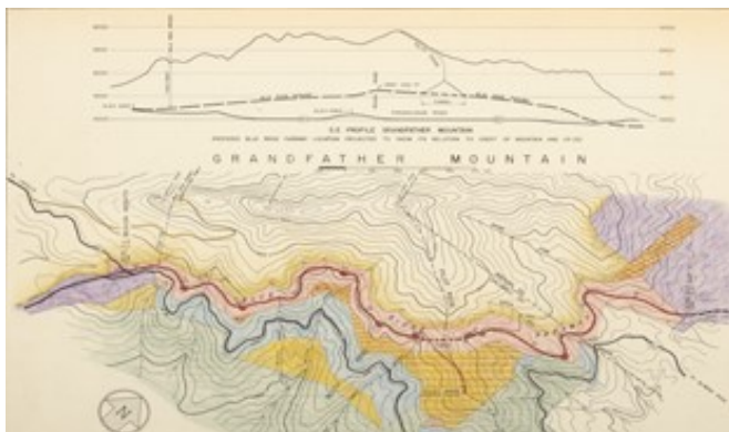
Construction drawings of the Blue Ridge Parkway roadway alignment along Grandfather Mountain shows how the parkway was constructed and integrated into the landscape of the surrounding area
