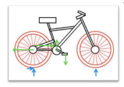
The frame divides the riders mass between both wheels. Larger wheels can increase the speed. Gears linked together by a chain increase the pedaling force. The pedal crank levers increase the pedal force. Spokes make the wheel strong and support the mass of the rider. The brake shoes apply friction to the rim to change energy into heat, which slows the bike down.
