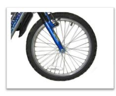
A wheel and an axle are a simple machine. The wheel will increase the force or speed depending on how it is turned. The greater the **diameter** of the wheel the more your speed can increase. Wheels support your mass as you sit on the seat. The rubber tire sits inside a wheel that has a rim and several **spokes**, which make the wheel strong, lightweight and help reduce the force of air resistance. Like strands of a spider web, the spokes are pulled tight
